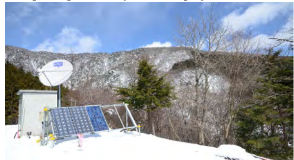
Figure 8. Data Communication System: Satellite Internet dish, solar panels, and control house in Cyber Forest project site.
